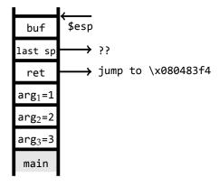
We need to fill this buffer over its limit of 8 characters so that it overwrites the stack pointer and then also overwrites the return address. If, for example, we want to jump to a specific address in memory, say, \x080483f4 then we can fill the buffer with the data
