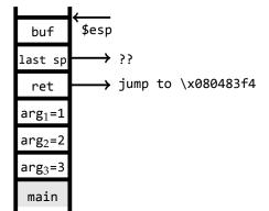
We need to fill this buffer over its limit of 8 characters so that it overwrites the stack pointer and then also overwrites the return address. If, for example, we want to jump to a specific address in memory, say, \x080483f4 then we can fill the buffer with the data
