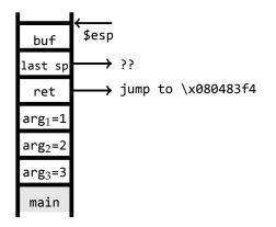
We need to fill this over its limit of 8 characters so that it overwrites the stack pointer and then overwrites the return address. If, for example, we want to jump to a specific address in memory, say, \x080483f4 then we need to fill the buffer for example as follows
