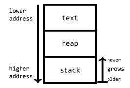
The text region contains the program code (usually this region is read-only). The heap stores all data the programmer explicitly allocates. For us the most interesting region is the stack, which contains data mostly associated with the control flow of the program. Notice that the stack grows from a higher addresses to lower addresses. That means that older items on the stack will be stored behind, or after, newer items. Let's look a bit closer what happens with
