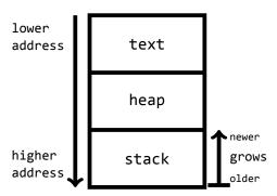
The text region contains the program code (usually this region is read-only). The heap stores all data the programmer explicitly allocates. For us the most interesting region is the stack, which contains data mostly associated with the control flow of the program. Notice that the stack grows from higher addresses to lower addresses (i.e. from the back to the front). That means that older items on the stack will be stored behind, or after, newer items. Let's look a bit closer
