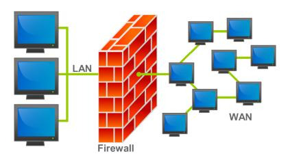
A firewall is a piece of software that controls incoming and outgoing traffic according to some rules.
