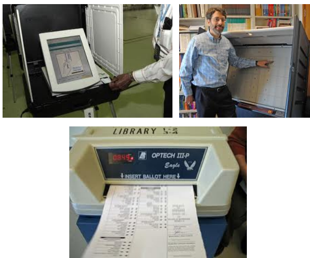
Figure 1: Direct-Recording Electronic voting machines above; an optical scan machine below.
