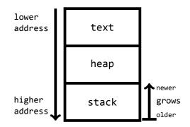
The text region contains the program code (usually this region is read-only). The heap stores all data the programmer explicitly allocates. For us the most interesting region is the stack, which contains data mostly associated with the control flow of the program. Notice that the stack grows from higher addresses to lower addresses (i.e. from the back to the front). That means that older items on the stack will be stored behind, or after, newer items. Let's look a bit closer
