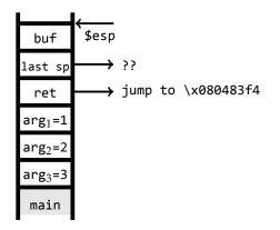
We need to fill this buffer over its limit of 8 characters so that it overwrites the stack pointer and then also overwrites the return address. If, for example, we want to jump to a specific address in memory, say, \x080483f4 then we can fill the buffer with the data
