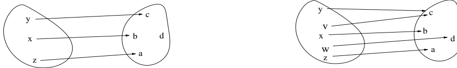
Figure 1.5: The function on the left is injective, but not surjective. The function on the right is surjective but not injective.
