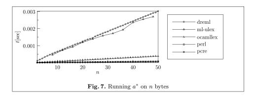
Figure 7 shows the timing results for matching a simple pattern against some large file. dreml and ml-ulex are comparable whereas ocamllex is much faster due to its C-based table engine. For comparison, we also include results for Perl and PCRE.
