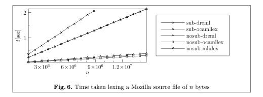
of include directives. As can been seen, for both cases performance results are comparable. This indicates that submatching generally does not incur any severe run-time penalty.
