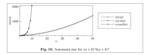
The exponential behavior of ocamllex and ml-ulex is due to the exponential size of the DFA automata. See Figure 10. In contrast, the NFA approach in dreml shows polynomial growth.
