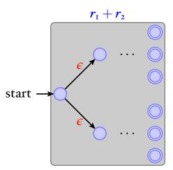
We (1) need to introduce a new starting state and (2) connect it to the original two starting states.
