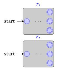
We (1) need to introduce a new starting state and (2) connect it to the original two starting states.
