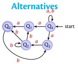
exchange initial / accepting states reverse all edges subset construction  $\Rightarrow$  DFA remove dead states
