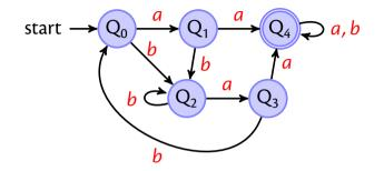
the start state can be an accepting state it is possible that there is no accepting state all states might be accepting (but this does not necessarily mean all strings are accepted)
