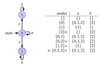
The nodes of the DFA are given by calculating all subsets of the set of nodes of the NFA (seen in the nodes column on the right). The table shows the transition function for the DFA. The first row states that  $\{\}$  is the sink node which has transitions for a and b to itself. The next three lines are calculated as follows:
