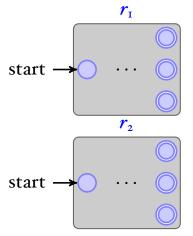
We (1) need to introduce a new starting state and (2) connect it to the original two starting states.
