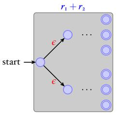
We (1) need to introduce a new starting state and (2) connect it to the original two starting states.
