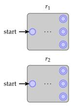
Each automaton has a single start state and potentially several accepting states. We obtain a NFA for the regular expression  $r_1+r_2$  by introducing a new starting state and connecting it with an  $\epsilon$ -transition to the two starting states above, like so
