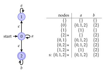
The nodes of the DFA are given by calculating all subsets of the set of nodes of the NFA (seen in the nodes column on the right). The table shows the transition function for the DFA. The first row states that  $\{\}$  is the sink node which has transitions for *a* and *b* to itself. The next three lines are calculated as follows:
