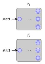
Each automaton has a single start state and potentially several accepting states. We obtain a NFA for the regular expression  $r_1 + r_2$  by introducing a new starting state and connecting it with an  $\epsilon$ -transition to the two starting states above, like so
