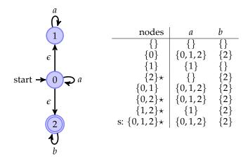
The nodes of the DFA are given by calculating all subsets of the set of nodes of the NFA (seen in the nodes column on the right). The table shows the transition function for the DFA. The first row states that  $\{\}$  is the sink node which has transitions for a and b to itself. The next three lines are calculated as follows:
