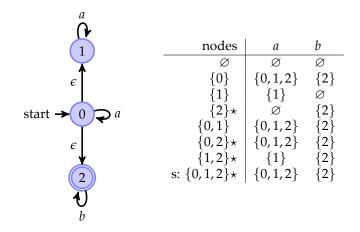
The nodes of the DFA are given by calculating all subsets of the set of nodes of the NFA (seen in the nodes column on the right). The table shows the transition function for the DFA. The first row states that  $\emptyset$  is the sink node which has transitions for *a* and *b* to itself. The next three lines are calculated as follows:
