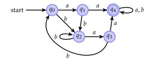
In this graphical notation, the accepting state  $q_4$  is indicated with double circles. Note that there can be more than one accepting state. It is also possible that a DFA has no accepting states at all, or that the starting state is also an accepting state. In the case above the transition function is defined everywhere and can be given as a table as follows:
