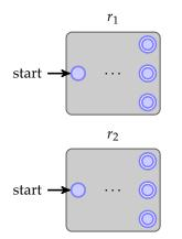
Each automaton has a single start state and potentially several accepting states. We obtain a NFA for the regular expression  $r_1 + r_2$  by introducing a new starting state and connecting it with an  $\epsilon$ -transition to the two starting states above, like so
